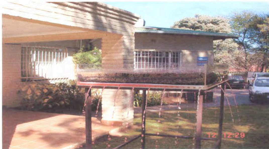
Figure 2: Drainage through the system one minute after commencement of the test
