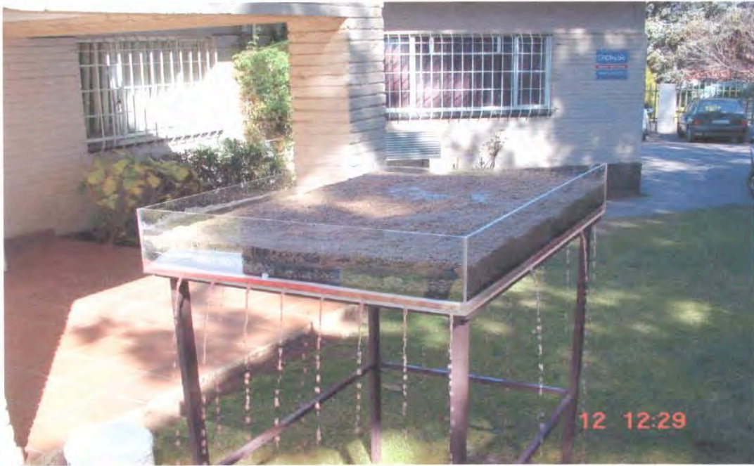
Figure 3: Drainage through the system two minutes after commencement of the test
